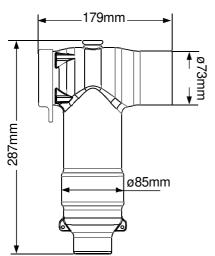
630A Series (*Tee Configuration*) follow IEC 60502-4 Connection Interface C follows EN50180 & 50181
